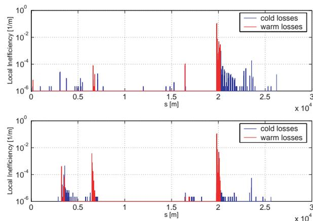
Figure 3: Example of proton losses in the LHC aperture along the LHC ring, for a vertical halo tracked at injection optics; Top: Only betatron cleaning (IR7) is considered; Bottom: The full LHC collimation system is considered.
