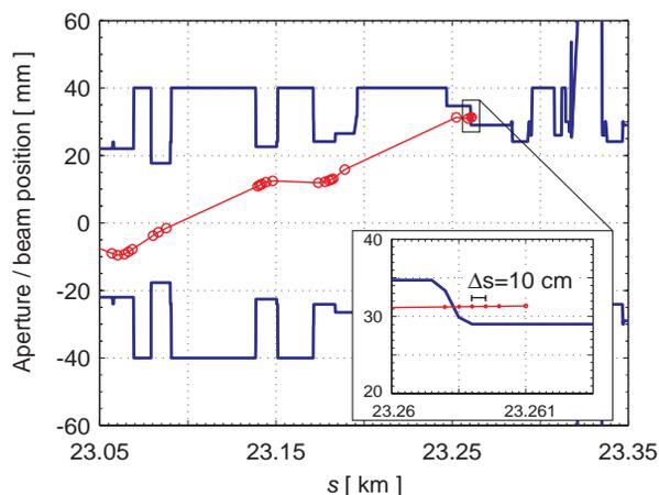
Figure 2: Example of a halo particle (red line) that hits the LHC aperture (blue line) [10].
