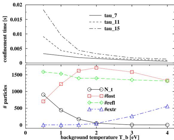
Figure 3: Number of trapped particles  $N_t$  after  $t_s = 10$  ms (and in the upper panel, confinement times  $\tau_i$  for charge states  $i$ ) vs  $T_b$ . Here  $N = 3200$ ,  $\Phi_1 = 0.89$  V,  $i_i = 1$ , initial kinetic energy  $E_i = eV_s + 2$  eV with source potential  $V_s = 12$  kV, position  $\mathbf{x}_i = (1, 4, -190)$  mm, ECR plasma in  $|z| < 138$  mm with ion temperature  $T_b = 1.5$  eV.
