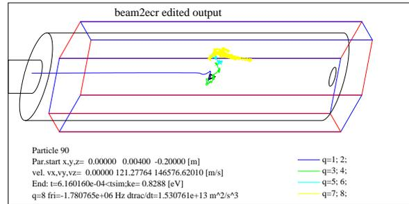
Figure 1: Track of a  $^{107}\text{Ag}$  ion, starting with charge  $i_i = 1$ ,  $E = 12003$  eV and stopping with  $i = 8$  at walls; source potential  $V_2 = 12$  kV; hexapole inner faces shown
