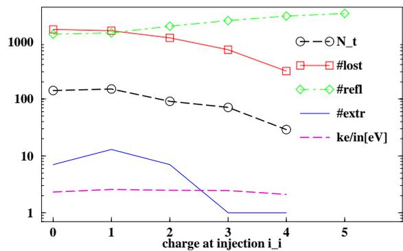
Figure 4: Number of trapped particles after  $t_s = 10$  ms vs  $i_i$  (fast neutral or ions) with initial kinetic energy  $E_i = i_i e(V_b + V_s) + 1$  eV with bias  $V_b = 1$  V; other condition as in Fig. 3. With  $i_i = 5$  all the 3200 particles are reflected.
