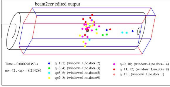
Figure 2: Trapped  $^{107}\text{Ag}$  ions, starting with  $i_i = 1$ ,  $N = 160$ ,  $V_b = 3$  V,  $V_s = 12$  kV,  $t_o = 0.298$  ms
