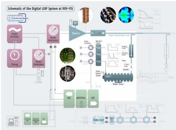
Figure 1: Schematic of the Digital RF Control System at 1.3GHz. It switches the LO phase by 90 degrees every microsecond. Digital I/Q detectors are used for the cavity field, and the incident and reflected waves. The digital boards are generic and flexible enough to be usable for a variety of control and data processing applications.
