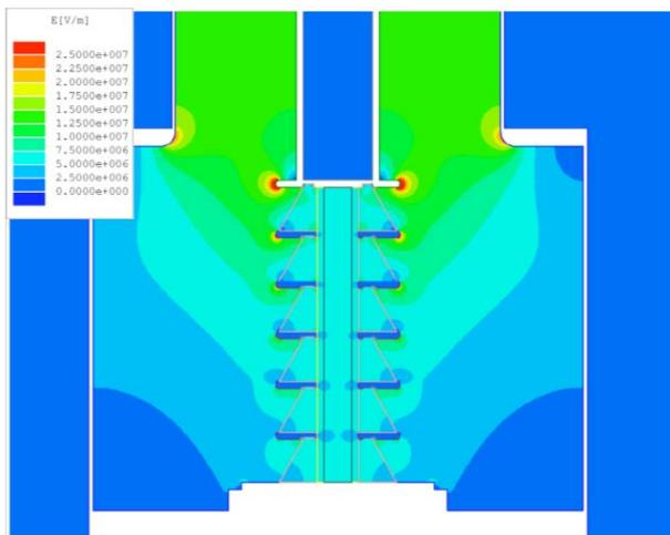
Figure 9: Configuration with the rounded corner in the junction of two MITL chambers.
