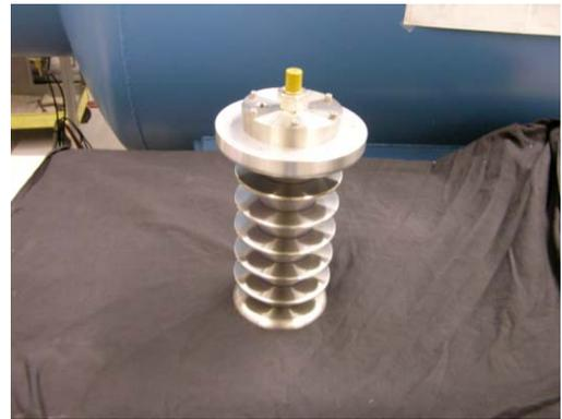
Figure 10: An insulator based on this design was fabricated.
