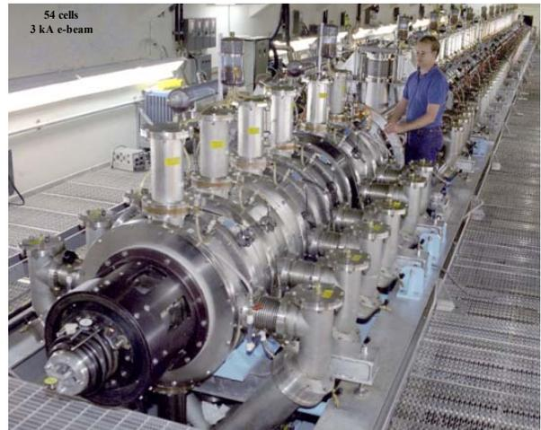
Figure 1: The FXR induction linac at LLNL.
