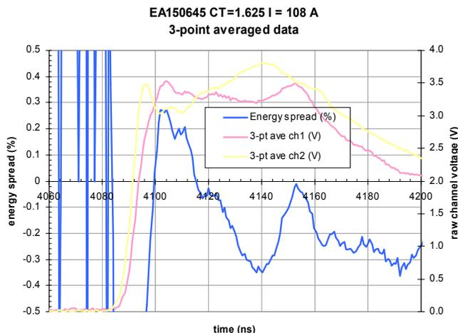
Figure 6: Initial results of the FXR Wire Scatter Energy Analyzer. The pulse is taken from 4100-4160 ns.
