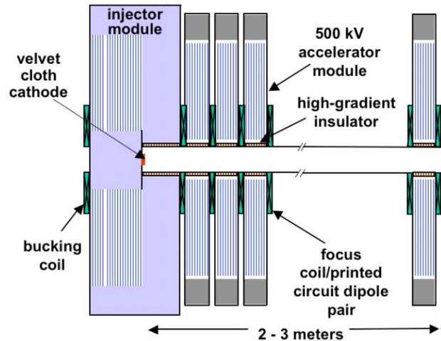
Figure 1: Dielectric wall induction accelerator configuration.
