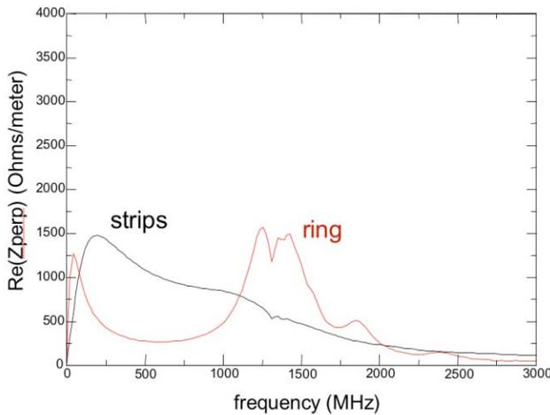
Figure 3: A 5-inch DWA stack simulated as a ring and as a strip
