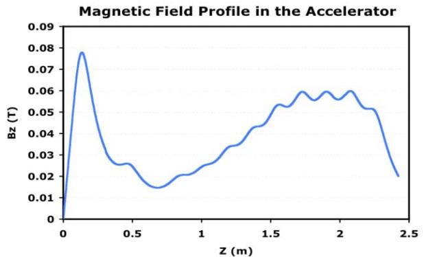
Figure 5: Optimized magnetic field profile for the 7.75-MeV beam
