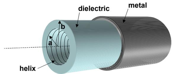
Figure 1: Schematic of helix, dielectric sleeve and outer conductor.
