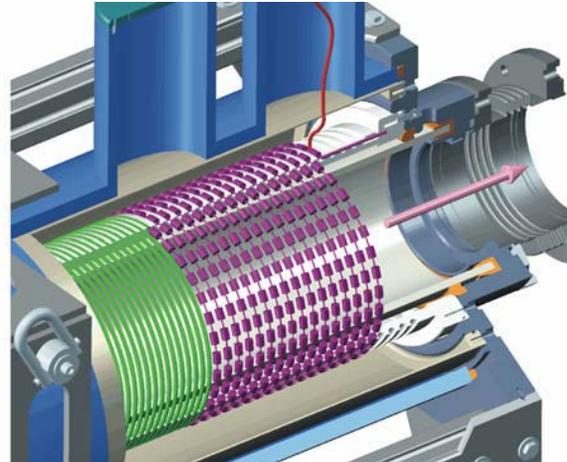
Figure 2: Termination resistor string for the oil dielectric helix.
