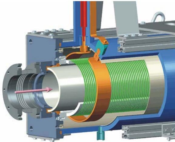
Figure 1: Transformer coupling with single turn primary strap on the oil dielectric helix.
