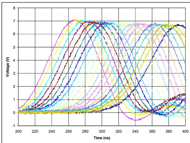
Figure 4:  $V(z,t)$  directly measured along helix at 1" intervals with air dielectric.
