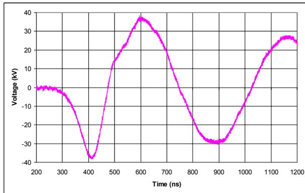
Figure 6: Initial high voltage waveform on the oil dielectric helix.
