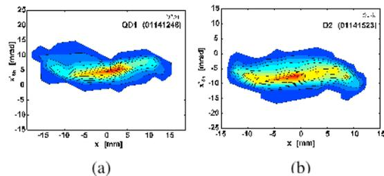
Figure 3. Horizontal phase-space diagrams (a) before and (b) after the electrostatic transport section for the 80% fill factor case ( $\Delta t = 0.12 \mu\text{s}$  at mid-pulse). Emittance is  $0.48 \pi \text{ mm-mrad}$  for both (a) and (b).
