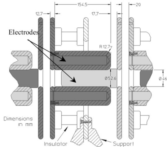
Figure 1: An HCX electrostatic quadrupole
