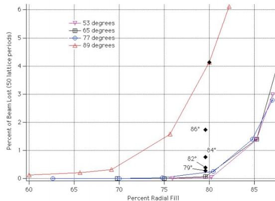
Figure 2. Beam loss in 50 focusing periods vs. radial filling factor for various values of  $\sigma_0$ .
