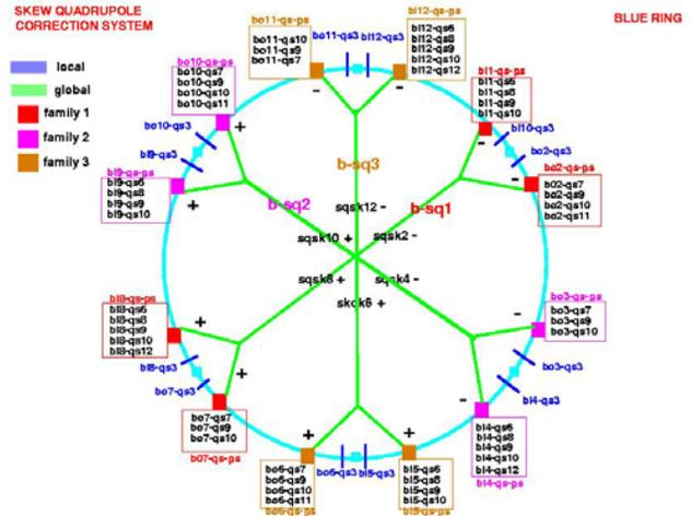
Figure 1: the schematics of the skew quadrupole families in the RHIC Blue ring. The configuration in the yellow ring is the same.
