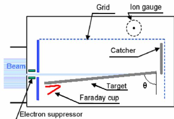
Figure 1: Gas-electron source diagnostic (GESD).
