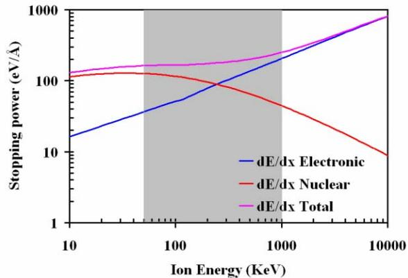
Figure 2: Stopping power for K<sup>+</sup> ions hitting Stainless Steel target.
