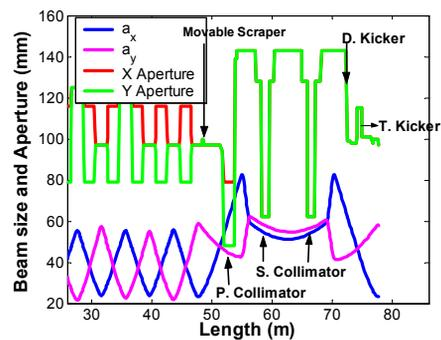
Figure 2: Beam pipe' aperture and beam size at the collimator region.
