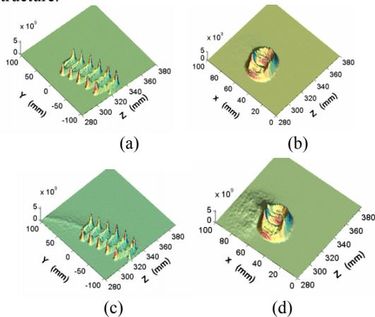
Figure 8: Distributions of electron cloud with a carbon (a)(b), and a copper (c)(d) catcher.
