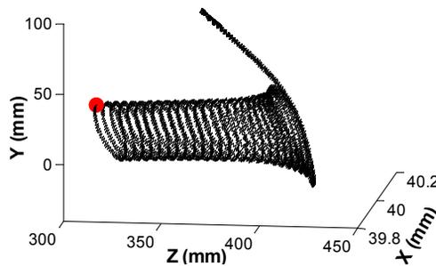
Figure 9: The orbit of a trapped electron. The electron is emitted from the foil at the peak of the beam’s profile. It hits the beam’s pipe at the bunch tail. The red dot is its emission position, the circulating-beam is in +Z direction.
