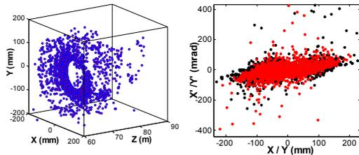
Figure 3: Distribution of lost particles at the secondary collimator.
