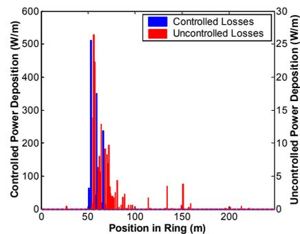
Figure 1: Power deposition along the ring.
