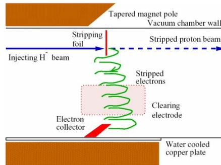
Figure 6: Collection of stripped electrons during the injection of the H- beam at the SNS ring. The foil is placed in a dipole magnet, which is part of the injection bump. The low pole surface of the magnet is extended downstream by about 20 cm so that the electrons are guided down to the electron collector.
