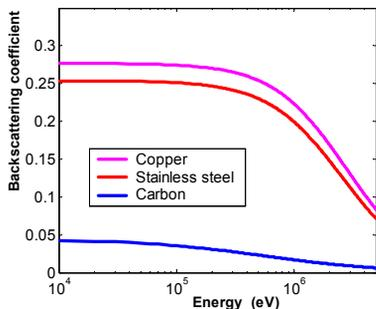
Figure 7: Backscattered electron coefficient of catchers of carbon, stainless steel, and copper with normal incidence electrons.
