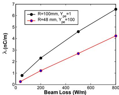
Figure 5: Effects of different pipe apertures on beam loss, R is the radius of beam pipe and  $Y_{pe}$  is the proton electron yield.
