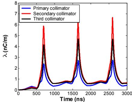
Figure 4: Electron build-up inside the collimators with a proton-electron yield of 100.
