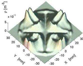
Figure 2: Distribution of the electrons in the quadrupole at 40ns after the last bunch in the train passed the electron cloud.
