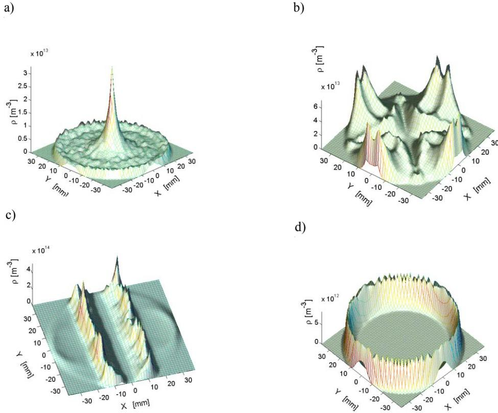
Figure 1: Distribution of the electrons in various places in the ring; a) drift space, b) quadrupole magnet, c) dipole magnet, d) solenoid.
