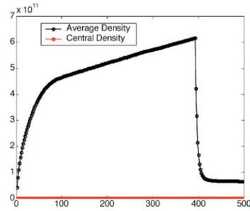
Figure 3: Average electron density and the electron density at the center of the chamber inside the solenoid in  $m^{-3}$ . Horizontal axis is time along the train in unit of ns. Even 400ns after the train passed the electron cloud some electrons are trapped.
