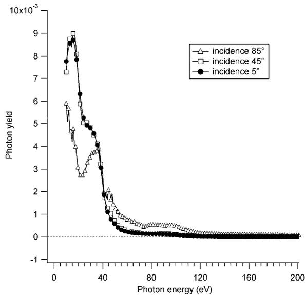
Figure 6: Photoelectron yield of the Al sample measured at incidence angles  $85^\circ, 45^\circ, \text{ and } 5^\circ$ .
