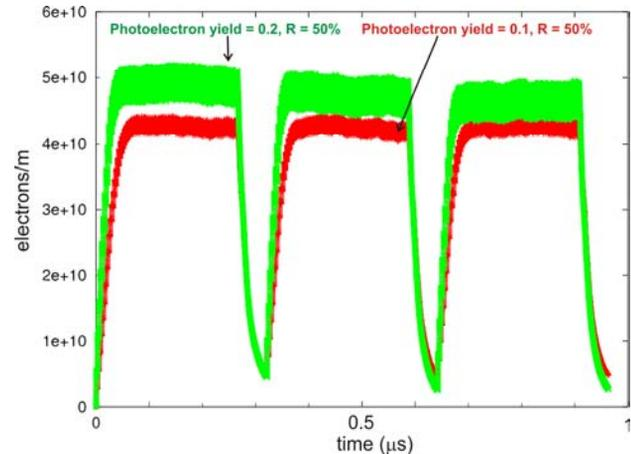
Figure 1: mean e-cloud linear density in the storage ring calculated for two different photoelectron yield values (0.2 and 0.1) with a reflectivity of 50%.
