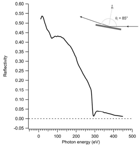
Figure 3: Reflectivity measurement with an incidence angle of  $85^\circ$ .
