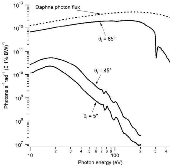
Figure 5: Number of reflected photons obtained by the reflectivity curves at incidence angle  $\theta_i = 85^\circ, 45^\circ, 5^\circ$ .
