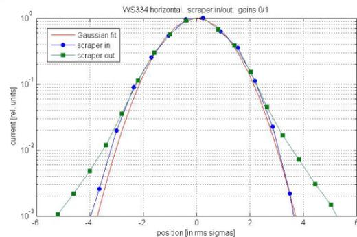
Figure 3: Effect of the MEBT scraper on the beam profile measured in the DTL. Blue circles – scraper is in; green squares – scraper is out; solid red line – Gaussian fit.
