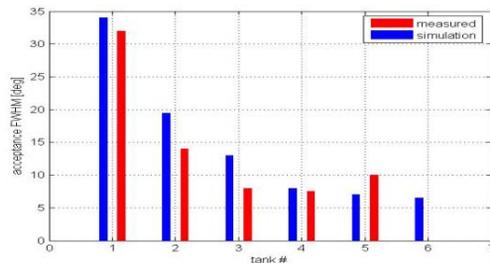
Figure 7: The measured (red) and simulated (blue) widths of the DTL acceptance curves vs. the tank number.
