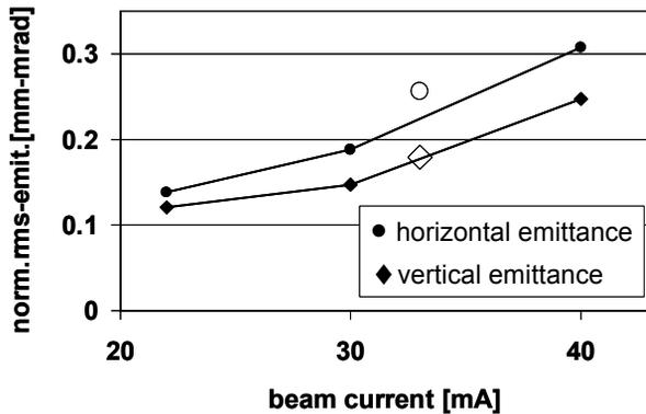
Figure 1: LEBT output emittance measurement results.
