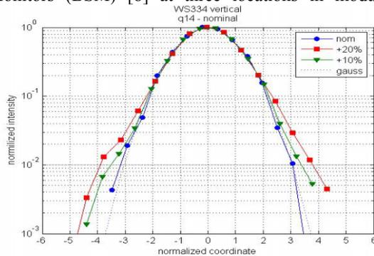
Figure 4: Effect of the MEBT matching quad change on the beam profile measured in the DTL. Blue circles – nominal “best match”; green triangles – nominal +10%; red squares – nominal +20%; dash – Gaussian fit.
