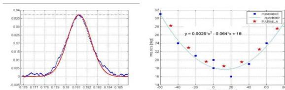
Figure 5: Left: longitudinal bunch profile measured with a mode-locked laser in the MEBT (blue) and Gaussian fit (red). Right: rms bunch length vs. the rebuncher phase: measurements – squares; simulation – stars; solid line – quadratic fit.
