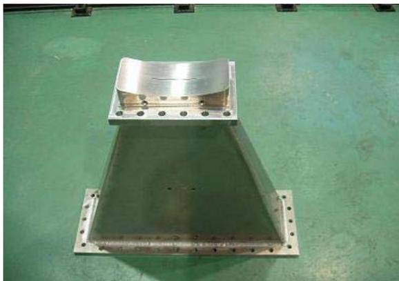
Figure 3: aluminium cold model iris coupler with ridge-loaded waveguide.
