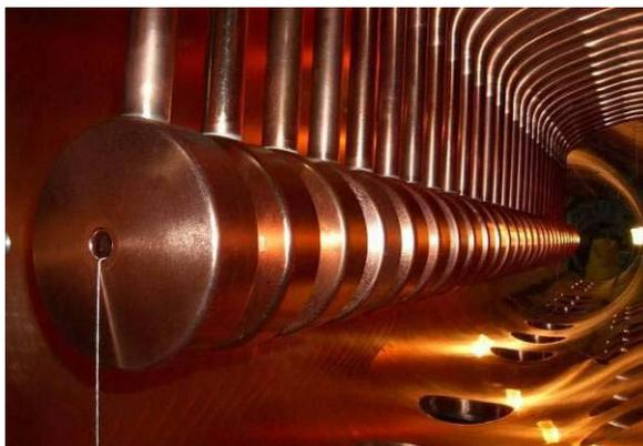
Figure 7: The aligned drift tube in the tank.
