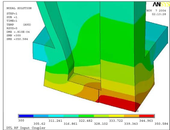
Figure 4a: Temperature distribution on the iris coupler.
