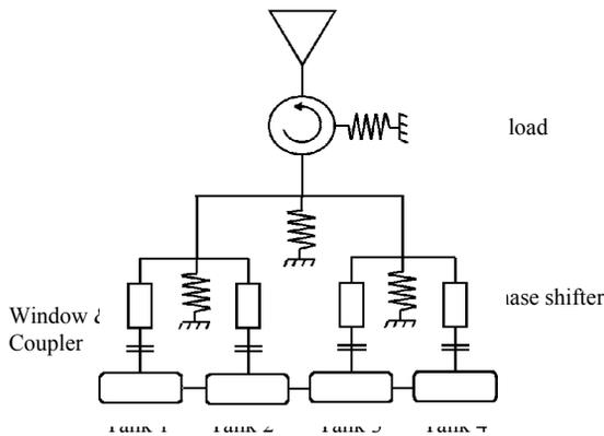
Figure 2: Schematic of RF power delivery system.
