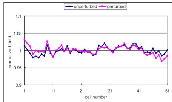
Figure 8: Tank1 field profile after tuning process.
