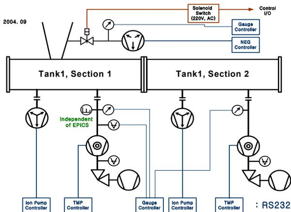
Figure 5: Vacuum System layout for PEFP DTL.
