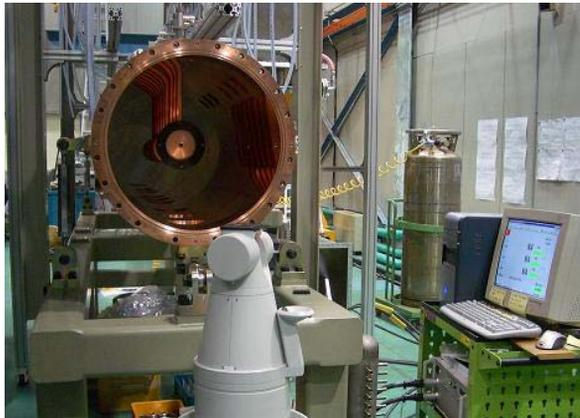
Figure 6: Drift tube alignment setup.
