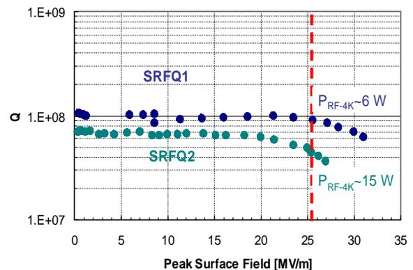
Figure 2: SRFQ1 and SRFQ2 Q performance. The curve is lowered by the presence of the normal conducting loop of the VCX fast tuner, which provides good phase stability of the resonators.
