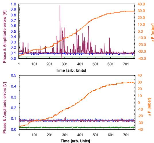
Figure 3: A 40 min sample of the stability behaviour (in phase and amplitude) of the SRFQs is shown. The pressure variation (orange curve) shows that  $\Delta P/\Delta t \leq 2$  mbar/min, i.e., better than specified.
