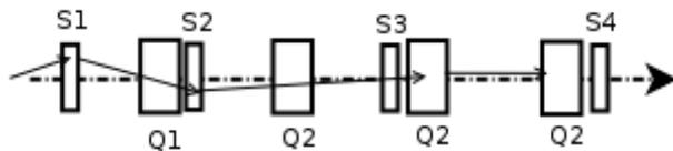
Figure 2: Schematic representation of the injection line with steering elements S1-S4 and quadrupoles Q1-Q4. The ideal beam line is shown as the dotted line.
