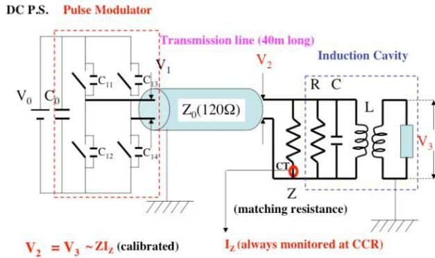
Figure 1. Equivalent circuit for the induction acceleration system
