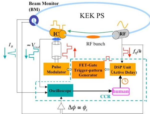
Figure 3. Schematic view of the hybrid accelerating system of the KEK PS
