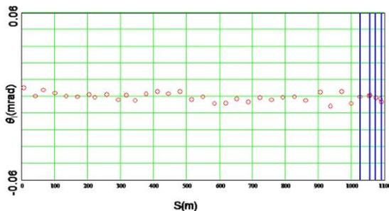
Figure 6: Kick strengths calculated from the orbit difference between MI at 150 GeV with LAM52 and V701 ramping and MI at 8 GeV after the LAM52 and V701 magnet bus work. The blue lines indicate the location of simulated kicks.
