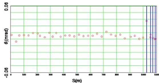
Figure 4: Kick strengths calculated from the orbit difference between MI at 150 GeV with LAM52 and V701 ramping and MI at 8 GeV before the LAM52 and V701 magnet buss work.. The blue lines indicate the location of simulated kicks.
