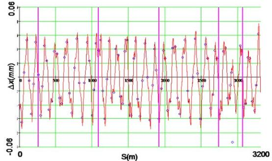
Figure 3: Orbit difference between MI at 150 GeV with LAM52 and V701 ramping and MI at 8 GeV before the LAM52 and V701 magnet buss work. Blue circles are measured values, red line is the fitted value. BPMs from RR-302 to RR-308 are masked. Note here most measured values of those BPMs are out of range.
