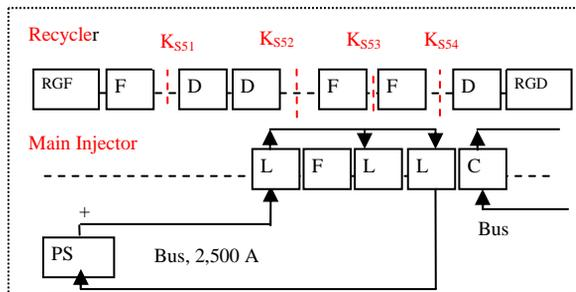
Figure 1: The lattice in Recycler ring around one of the Main injector Lambertson (L) and C-magnet (C). RGF and RGD represent the gradient magnets, F and D represent focusing and defocusing quadrupoles. PS is Power Supply.  $K_{s51}$ ,  $K_{s52}$ ,  $K_{s53}$  and  $K_{s54}$  (in red) are simulated virtual kicks.
