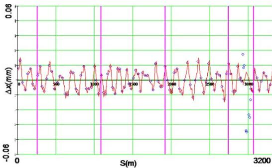
Figure 5: Orbit difference between MI at 150 GeV with LAM52 and V701 ramping and MI at 8 GeV after the LAM52 and V701 magnet bus work. Blue circles represent measured values, red line is the fitted value.
