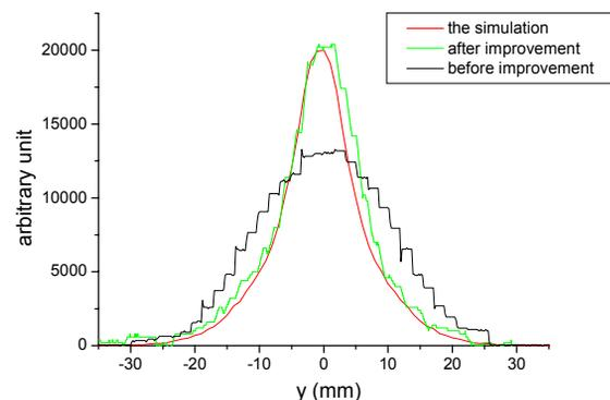
Figure 2: The vertical profile of the circulating beam. Black line is before the optimization and green line shows the beam profile with the new optics. Red line is beam distribution with the new optics by simulation.
