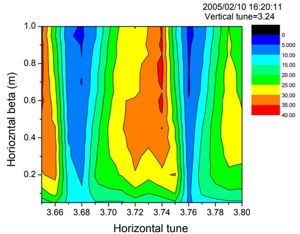
Figure 1: The multiturn-injection gain as both the functions of the horizontal tune and the horizontal beta function of the injection line at injection point.
