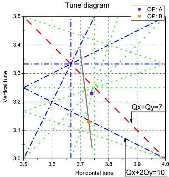
Figure 4: Tune diagram and measurement line of tune survey. Grey solid line: measurement line of tune survey, red dash: 2nd-order resonance line, blue dash dot: 3rd-order resonance line, green dot: 4th-order resonance line. Operation point (OP) A is  $(Q_x, Q_y)=(3.74, 3.23)$ , and operation point B is  $(Q_x, Q_y)=(3.73, 3.13)$ .
