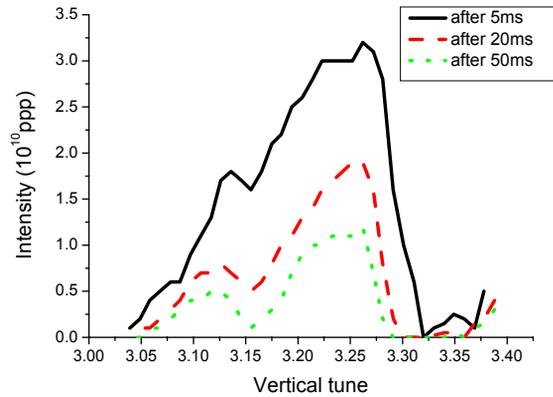
Figure 6: Intensity as a function of vertical tune when beam is bunched after 5ms (black solid line), 20ms (red dash line), and 50ms (green dot line).
