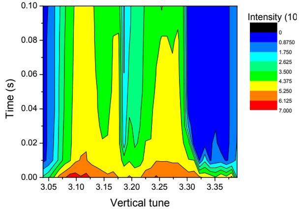
Figure 5: Intensity as a function of the vertical tune and time after injection.
