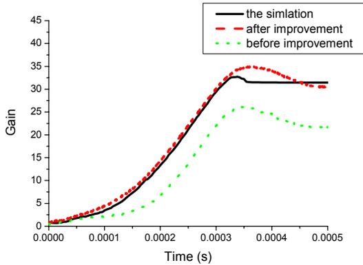
Figure 3: The injection gain during the multiturn injection and 500  $\mu$ s after the end of the injection. Black solid line: the gain by simulation. Red dash line: the gain after optimizations. Green dot line: the gain before optimizations
