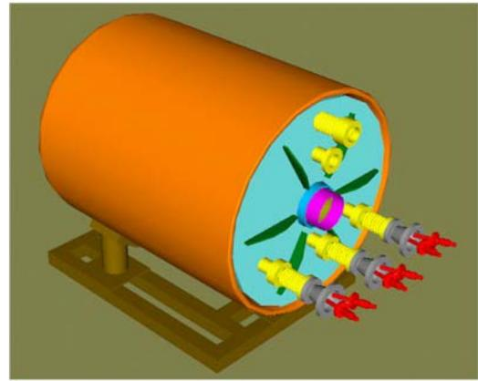
Figure 3: Design of the pulsed targetry magnet. The magnet has three nested coils that permit operation at 5, 10, and 15 T field. The magnet has a 15 cm warm bore and 1 m long beam pipe. The coils are normal conducting but cooled to liquid-nitrogen temperature to ease the requirements on the power supply.
