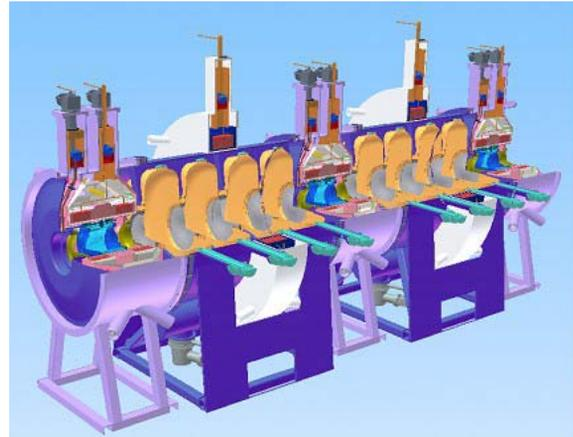
Figure 12: MICE cooling channel layout. There are two RF cavity and coupling coil (RFCC) modules and three absorber and focusing coil (AFC) modules.
