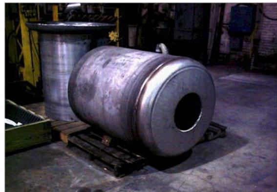
Figure 5: Cryostat pressure vessel for the targetry magnet.
