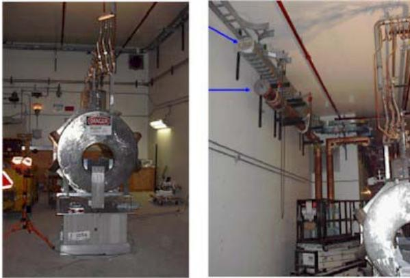
Figure 6: The 5-T superconducting magnet (left) and 805 and 201 MHz RF transmission lines (right) at the MTA.
