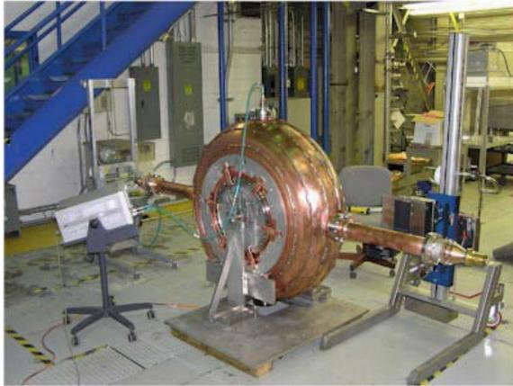
Figure 8: The 201 MHz prototype cavity with two RF couplers attached during a low power microwave measurement conducted at Jlab in March 2005.
