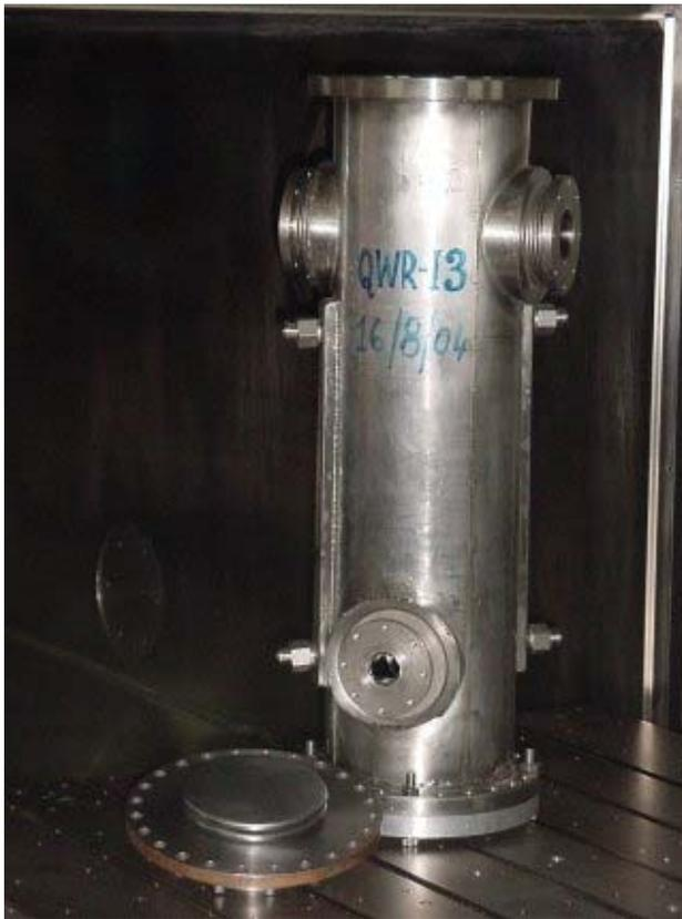
Figure 1: Indigenously built niobium quarter wave resonator with slow tuner bellows at NSC.
