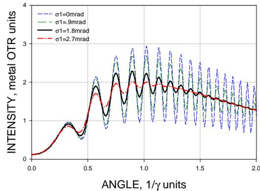
Figure 6: Effect of beam divergence on OTR-DOR interferences
