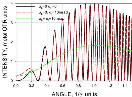
Figure 5: Effect of beam divergence on OTR-DOR interferences.
