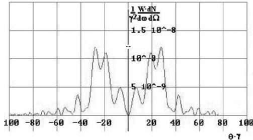
Figure 4: Parallel polarization component of backward ODR intensity from a slit of  $0.1\lambda\gamma$  width for  $\gamma$  at 60,000. Angular distribution in polarization plane, calculated with the pre-wave zone effect.
