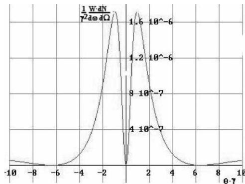
Figure 3: Parallel polarization component of backward ODR intensity from a slit of  $0.1\lambda\gamma$  width for  $\gamma$  at 60000. Angular distribution in polarization plane, calculated without accounting of the pre-wave zone effect.
