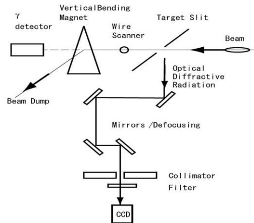
Figure 1: A schematic diagram of an ODR beam size monitor
