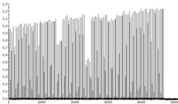
Figure 2: Wall current monitor for fill 3107, 110 bunches
