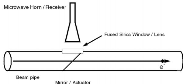
Figure 2: Microwave horn / detector arrangement used to detect coherent transition radiation. Plan view.
