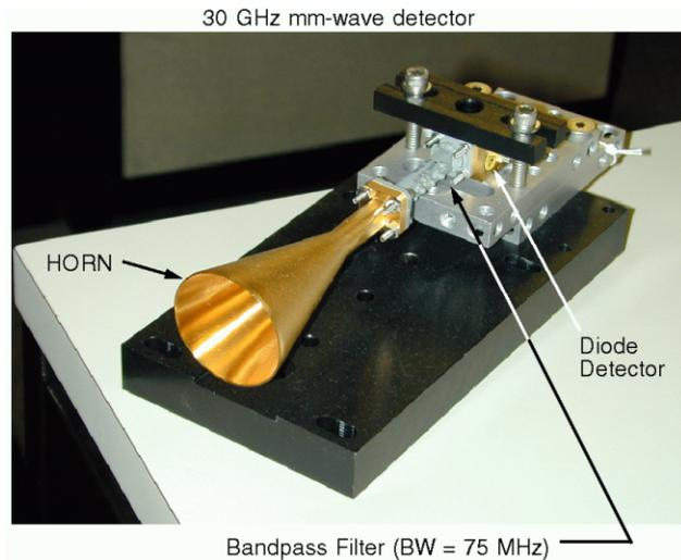
Figure 1: Microwave horn / detector assembly used to detect coherent transition radiation.
