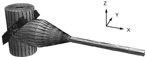
Figure 3: Microwave horn geometry used in MAFIA simulation.
