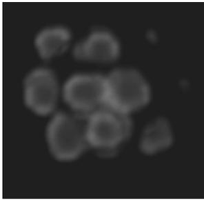
Fig. 3. Phosphor screen image downstream of the pepper pot showing a hollowed velocity space distribution.
