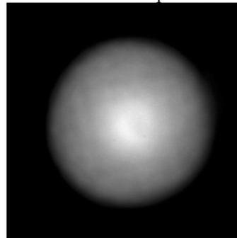
Fig. 1. Phosphor screen image of the beam approximately 60 mm from the anode plane. A weak shadow of the anode grid is observable.
