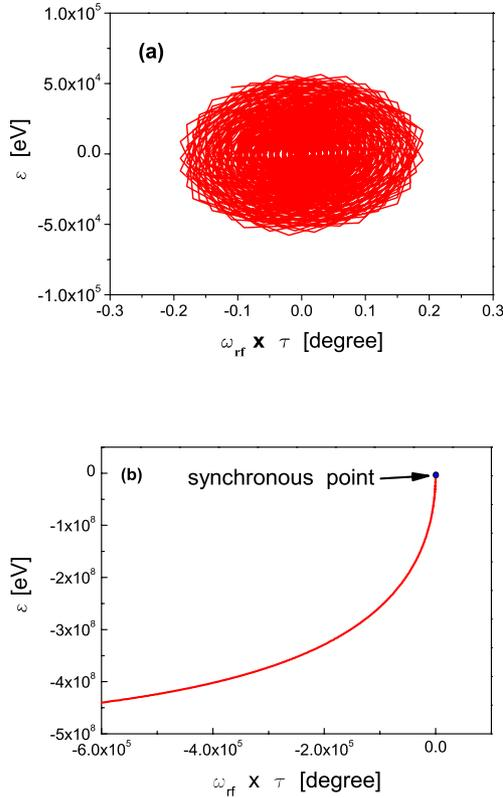
Figure 2: Simulated beam motion described by phase and energy deviations as beam current is (a) under or (b) above the maximum limit
