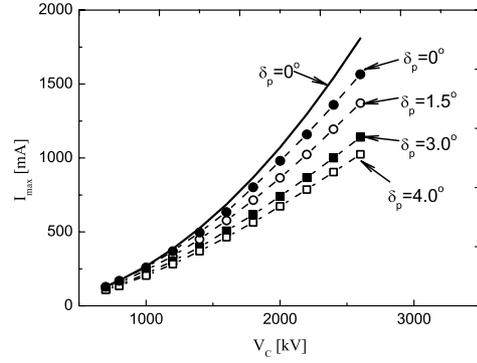
Figure 3: simulated maximum stored beam current versus the generator rf signal with different phase noise levels (symbol-dashed curves), and that predicted from (15) in the case of no noise (solid curve). The parameters used are  $E_s = 1.5 GeV$ ,  $\omega_{rf} = 500 MHz$ ,  $Q_0 = 1.0 \times 10^9$ ,  $R_s/Q_0 = 44.5$ ,  $\beta = 4000$ ,  $T_0 = 200/\omega_{rf}$ ,  $\alpha = 6.768 \times 10^{-3}$ ,  $\omega_p = 720 Hz$ ,  $U_{rad}(\varepsilon = 0) = 168 keV$ ,  $P_{loss} \equiv V^2/2R_s$ .
