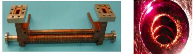
Figure 5. Damage in X-band structure.
