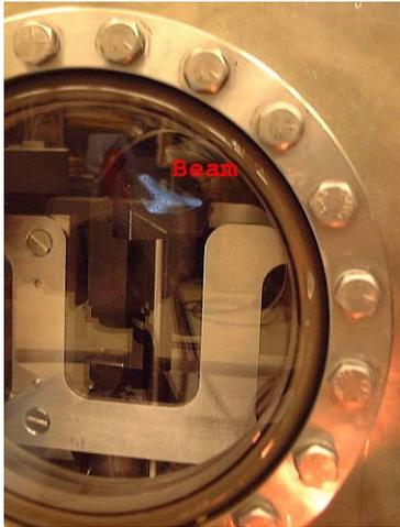
Figure 5: Beam intercepted in phosphor screen
