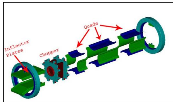
Figure 4: Quads, Chopper, Inflector Plates Section
