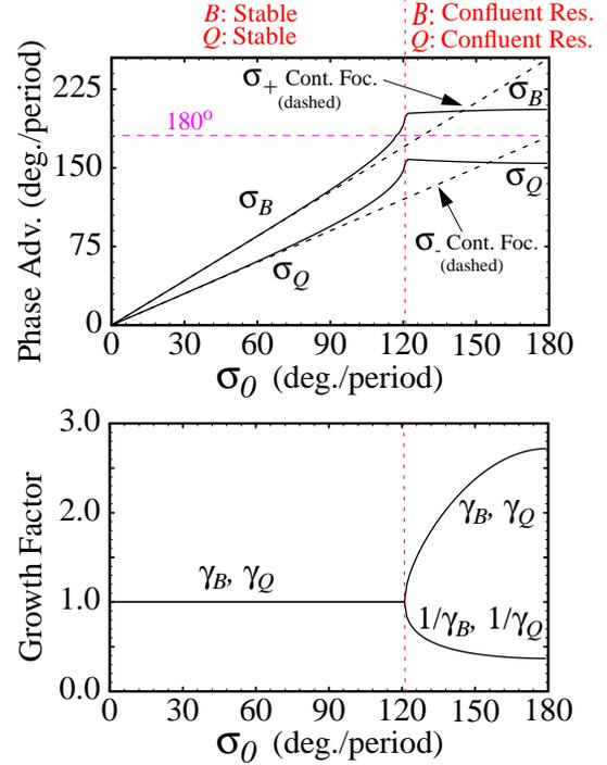
FIG. 3: Phase advance ( $\sigma_Q$  and  $\sigma_B$ ) and growth factors ( $\gamma_Q$  and  $\gamma_B$ ) for the breathing and quadrupole modes for a thin-lens FODO quadrupole focusing channel and a fully depressed beam. Continuous focusing model predictions for  $\sigma_{\pm}$  are superimposed (dashed curves).
