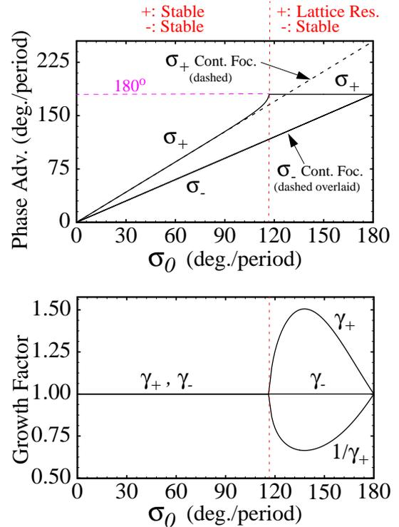
FIG. 2: Phase advances ( $\sigma_\pm$ ) and growth factors ( $\gamma_\pm$ ) for the breathing and quadrupole modes for a thin-lens solenoidal focusing channel and a fully depressed beam. Continuous focusing model predictions for  $\sigma_\pm$  are superimposed (dashed curves).
