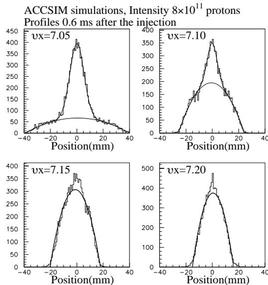
Figure 5: ACCSIM simulation of the horizontal beam profiles 0.6 ms after injection when the injection beam intensity was  $8 \times 10^{11}$  protons and the horizontal tune was 7.05, 7.10, 7.15 or 7.20.
