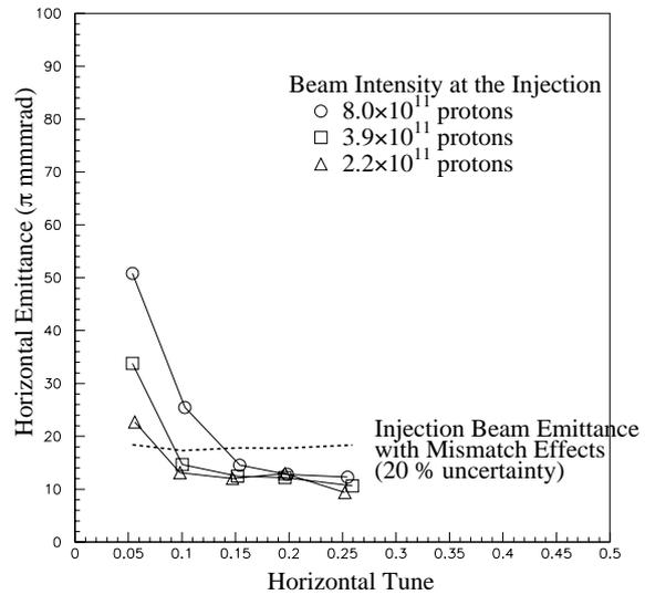
Figure 3: Horizontal 87% emittance as a function of the horizontal tune for the beam intensity of 2.2, 3.9 and  $8.0 \times 10^{11}$  protons.
