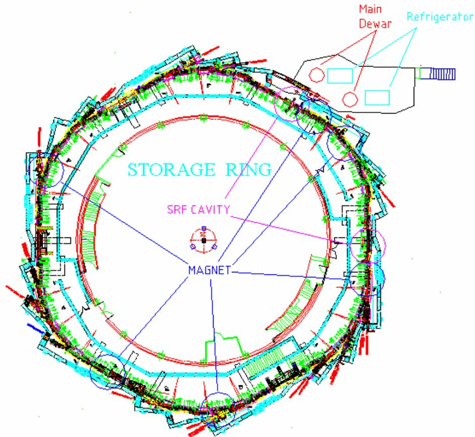
Figure 1: Locations of SRF cavities and SM modules.
