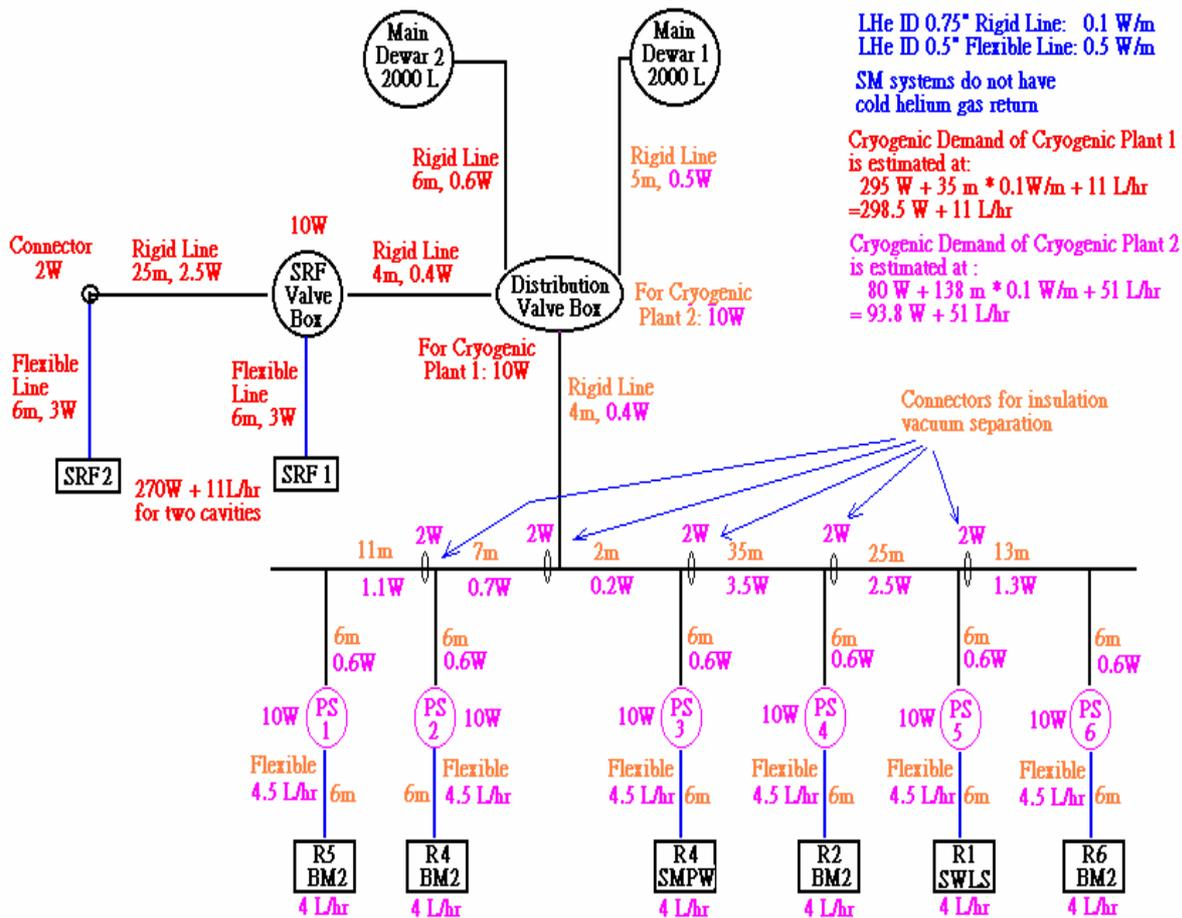
Figure 2: Estimated heat leak of SRF cavities, SM module, and associated valve boxes and piping.
