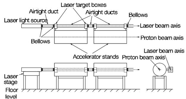
Figure 1: Conceptual view of the laser-based alignment system.
