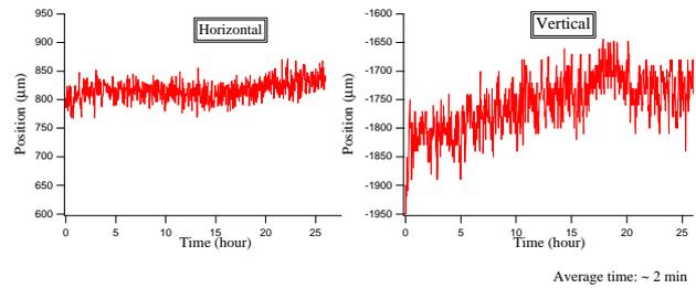
Figure 7: Time evolution of the photo-diode readout in a 100 m experiment.
