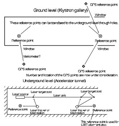
Figure 4: Determining of the laser axis.
