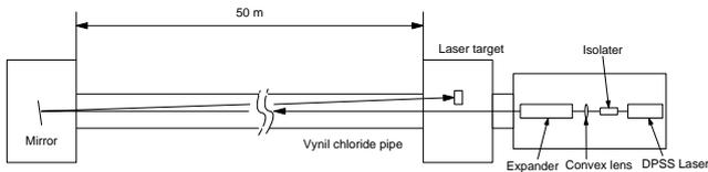
Figure 5: Conceptual view of the experimental setup.
