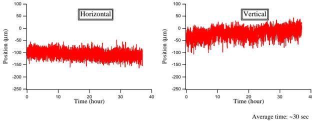
Figure 6: Time evolution of the photo-diode readout in a 50 m experiment.
