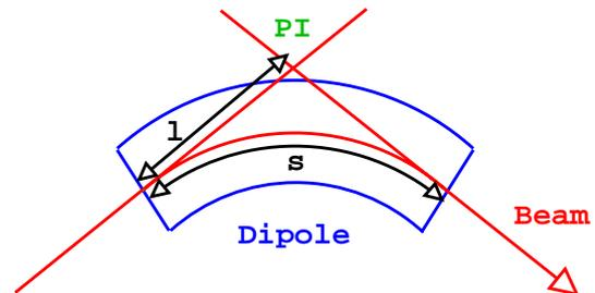
Figure 1: Schematic of the dipole showing the beam direction and the two intersecting tangents (PI). Fixing the PI point freezes the geometry.
