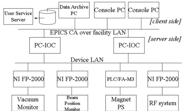
Figure1: Schematic drawing of the SAGA-SL control system
