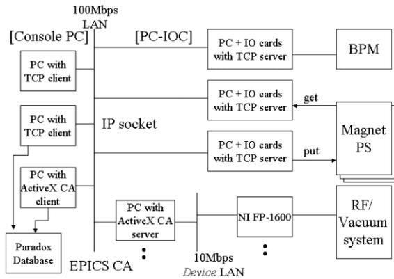
Figure 3: Block diagram of the AIST control system at the present stage.
