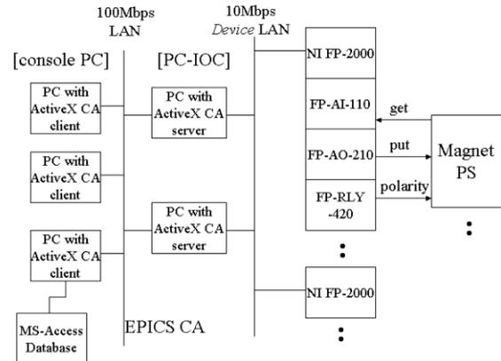
Figure 2: Block diagram of the IAE magnet control system.
