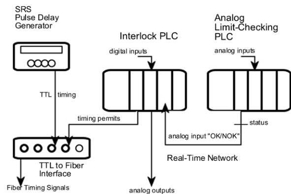
Figure 1: Linac Control System Architecture
