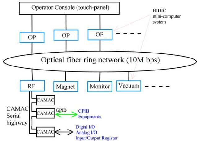
Figure 1: AR control system before the improvement (TRISTAN control system). "OP" denotes the HIDIC mini-computers for control of operator console.
