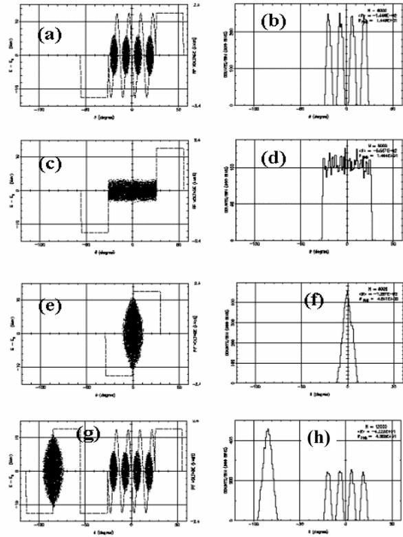
Figure 2. ESME simulations of the beam stacking in the Recycler. The figures (a), (c), (e) and (g) show  $(\Delta E, \Delta\theta)$ -phase space distributions of beam particles. The figures on right show their projections on  $\theta$  – axis (equivalent time coordinate).
