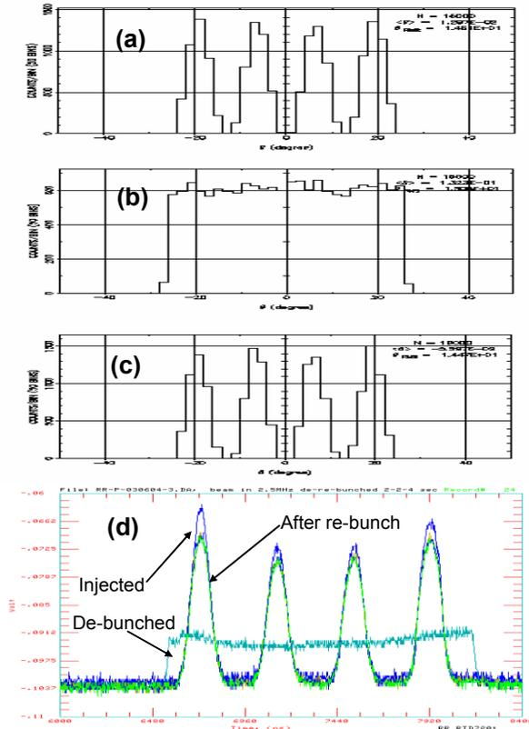
Figure 1. Results of ESME simulations of wall current monitor data. (a) The beam at injection in the 2.5MHz buckets, (b) De-bunched in 8 sec, (c) Re-bunched in 8 sec as explained in the text. (d) Wall current monitor data taken during a beam experiment for similar conditions. The measured bunch lengths before de-bunching and after re-bunching are essentially the same.
