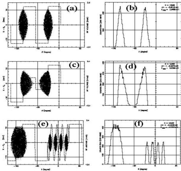
Figure 3. ESME simulations to illustrate a way of merging two stacks (particularly see (c) and (d)). (e) and (f) illustrate a new injection.
