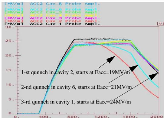
**Figure 3:** Quench detection during high gradient run at Module 1\*.
