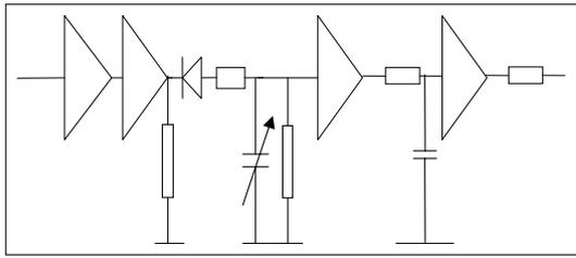
Figure 2 – Block diagram of the pulse treatment circuit.
