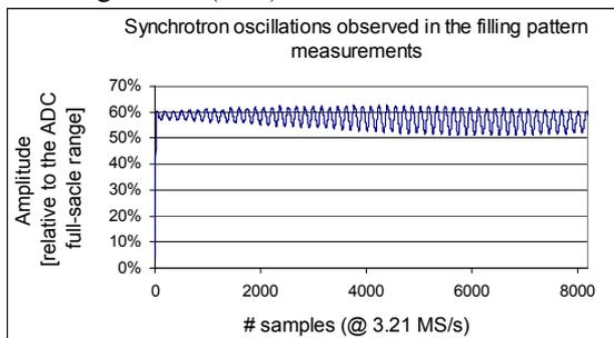
Figure 5 – 8-ksample acquisition of a signal of a 2 mA bunch.
