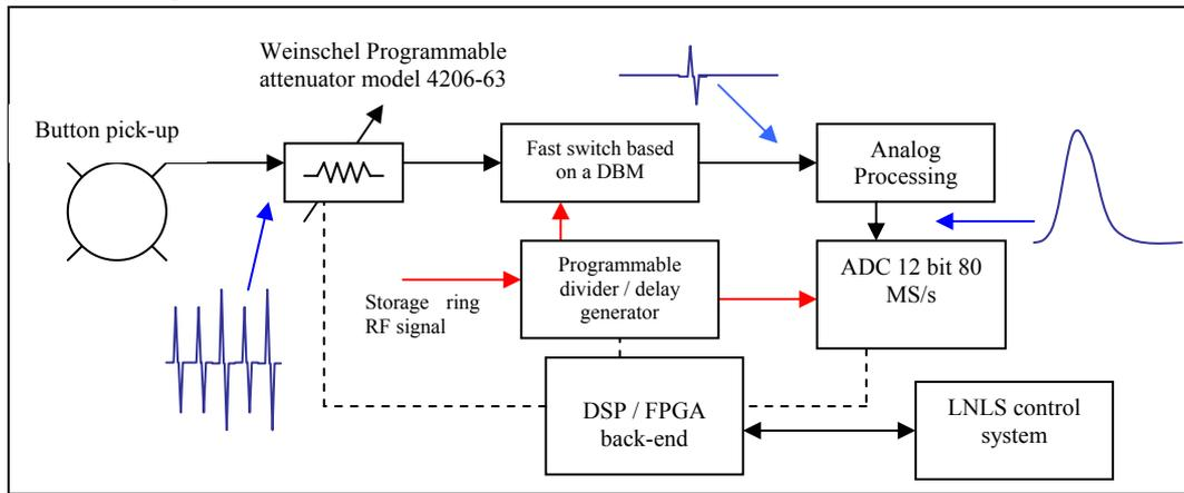
Figure 3: Block diagram of the bunch charge meter
