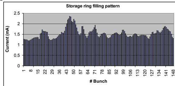
Figure 7 – Typical filling pattern of the storage ring.
