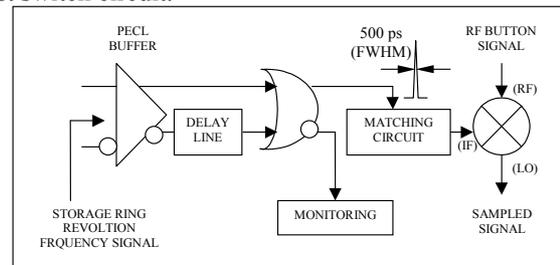
Figure 1 – Fast switch circuit.
