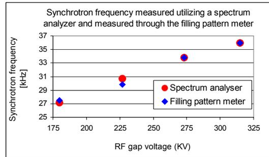
Figure 6 – Synchrotron frequency measured by utilizing a spectrum analyzer and the bunch charge meter (FFT).
