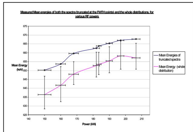
Fig. 3: Comparison of mean energies of truncated and untruncated spectra
