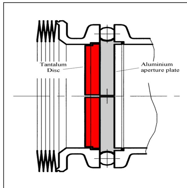
Fig. 1: The new tantalum disc attached to the aperture plate
