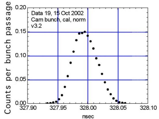
Figure 2. Beam intensity profile of a single bunch in the ALS measured by correlation of synchrotron light emission with a mode locked solid-state laser oscillator.
