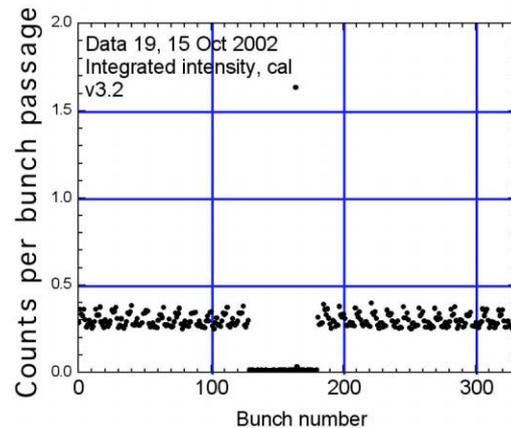
Figure 3. Integrated intensity of all 328 RF buckets in the ALS.
