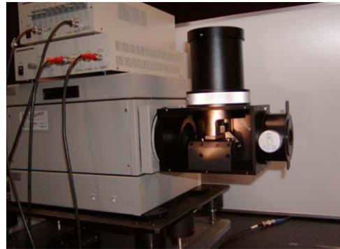
Figure 8: A photograph of the Offner-type relay system with the streak camera. The cover of the Offner-type relay system is opened to show the inside.
