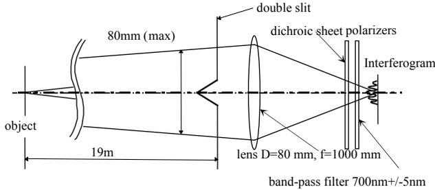
Figure 3: Aplanatic Fizeau type double-slit SR interferometer for the horizontal beam size measurement.
