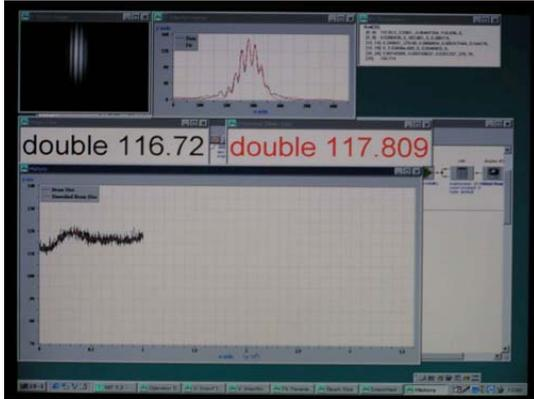
Figure 6: Display panel for automatic beam size measurement. This example shows a panel for vertical beam size measurement.
