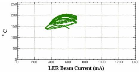
Figure 2: Old beam-pipe temperature dependence on beam current.
