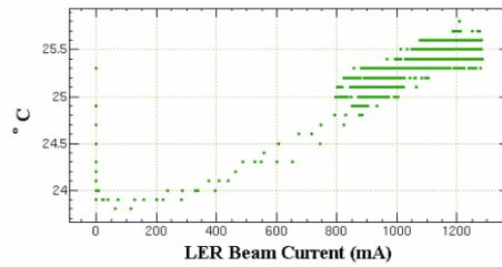
Figure 4: New beam-pipe temperature dependence on beam current.
