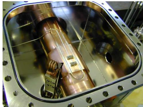
Figure 8: Inside of new LER synchrotron radiation extraction chamber, showing extraction mirror (lower left) and light-extraction aperture in outer chamber wall (middle right).
