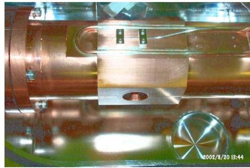
Figure 7: Inside of new LER synchrotron radiation extraction chamber, showing light extraction aperture in beam-pipe (center).
