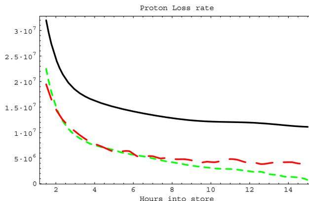
Fig. 1 Loss rate in protons/sec. vs. time in hours near the start of Store 2424. The solid curve is the total proton loss rate. The dotted curve is the loss rate after subtracting the losses due to luminosity, diffusion from the RF bucket, and collisions with the residual gas. The dashed curve is 25 times the E0LTOT counter rate.
