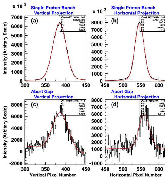
Figure 6: (a,b) Vertical and horizontal projections of the background subtracted image for a single  $1.8 \times 10^{11}$  proton bunch at normal MCP high voltage; (c,d) Vertical and horizontal projections of the background subtracted image for a 670 ns time interval in the beam abort gap. The projections are fit with a Gaussian signal and a linear background function.
