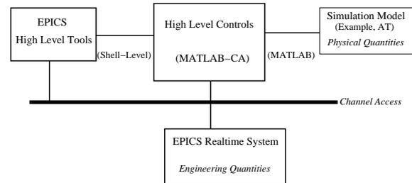
Figure 1: A layout of a typical integrated accelerator control system.
