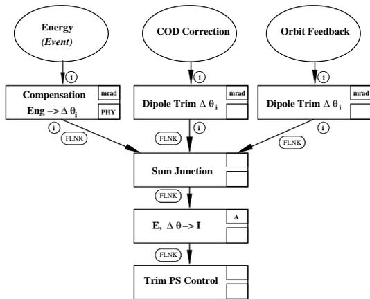
Figure 4: Multiple controls of a shared dipole trim.
