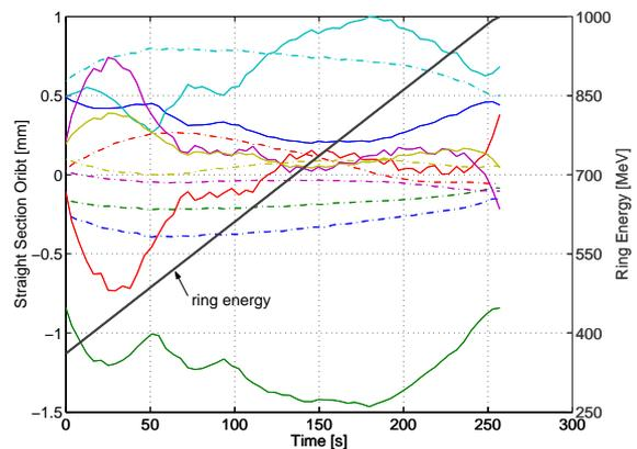
Figure 5: Beam orbit in the wiggler straight section during energy ramping. Solid and dot-dashed lines are horizontal and vertical orbits, respectively.
