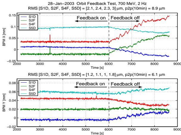
Figure 5: Orbit stability with a slow orbit feedback system. All 4 BPMs are located in the straight section with large  $\beta$ -functions.
