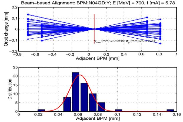
Figure 3: Finding the vertical quad center using a Gaussian fit for quad N04QD,  $\beta_y = 12$  m.
