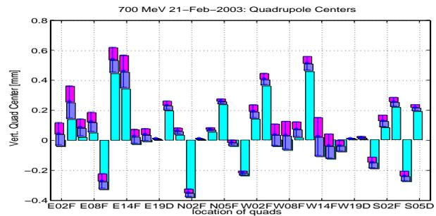
Figure 4: Measured vertical offsets between quad centers and adjacent BPM centers with a 700 MeV beam.
